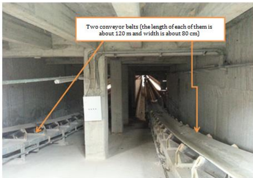
Figure 9 Conveyor Belt 1 Which is Located Inside the Bunker
